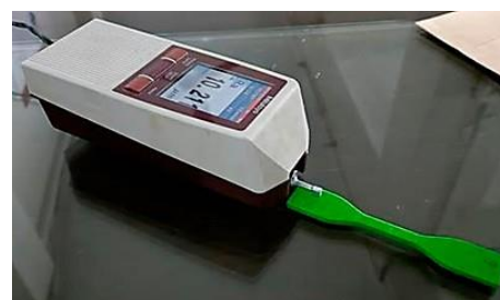
Figure 6. Surface roughness measurement using a Mitutoyo surface roughness tester.
