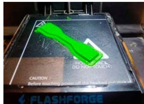
Figure 4. 3D printing of specimen on FlashForge 3D printer.
