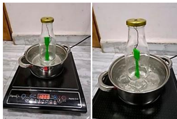
Figure 7. Vapor smoothing process using ethyl acetate solvent.
