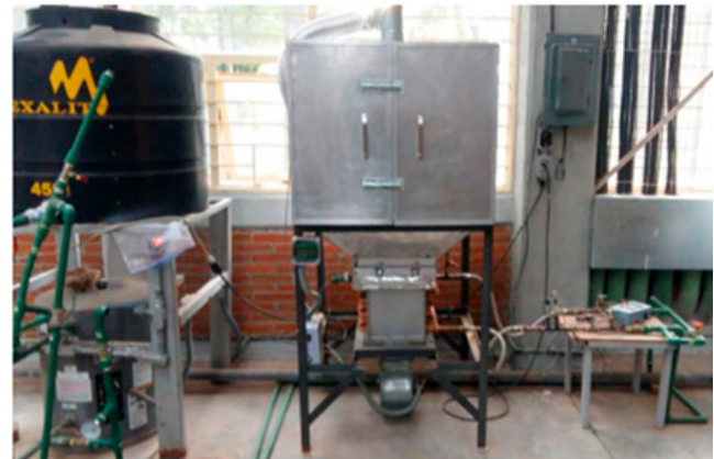
Figure 2. Geothermal dryer system laboratory prototype.
