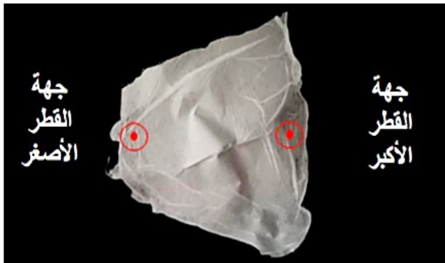
Figure 7. Method of selecting samples for microscopic examination.
