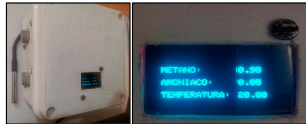
Figure 9. Functional prototype of the controller device.
