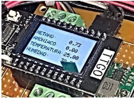
Figure 4. Controller measurement for sensor calibration.
