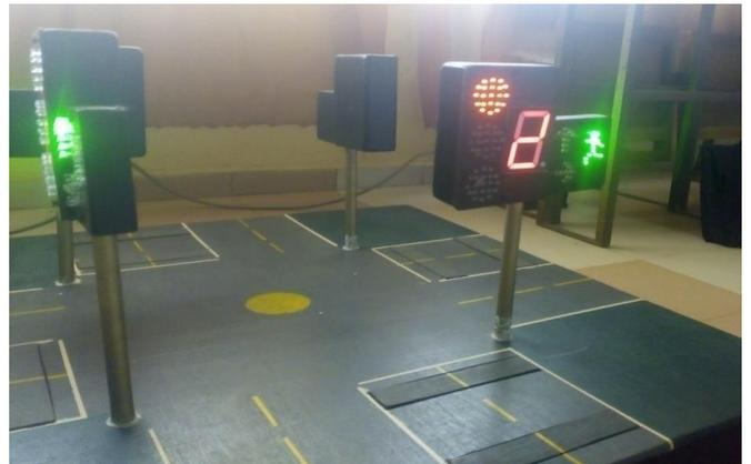
Figure 7. Diagram of the prototype giving right of way to road 1 pedestrians.
