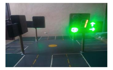
Figure 6. Diagram of the prototype giving right of way to road 1 motorists.
