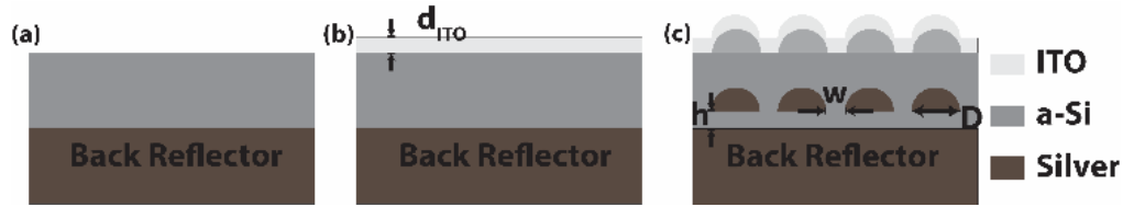
Fig. 1. Cross-sectional view of the device a) bare a-Si with Ag back reflector, b) ITO/a-Si/Ag back reflector, c) Hemispherical nanoparticle for plasmonic behavior (ITO/a-Si (hemispherical Ag nanoparticle)/Ag-back reflector).
