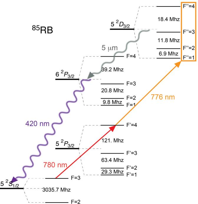
Figure 1. Energy-level diagram for the  $5\text{S}_{1/2} \rightarrow 5\text{P}_{3/2} \rightarrow 5\text{D}_{3/2}$  of atomic  $^{85}\text{Rb}$ , including the hyperfine states.
