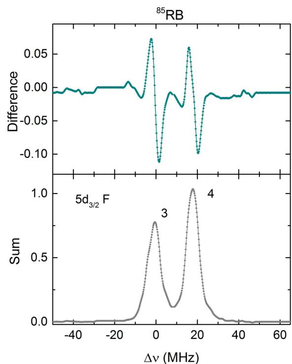
Figure 5. The polarization rotation (top) and the changes in the total absorption (bottom) induced in the 780 nm beam obtained with the 780 nm laser locked to the 5 S<sub>1/2</sub>, F = 3 → 5 P<sub>3/2</sub>, F' = 4 cycling transition of <sup>85</sup>Rb and the frequency of the 776 nm laser scanning across the resonances of the 5 P<sub>3/2</sub> → 5 D<sub>3/2</sub> manifold.
