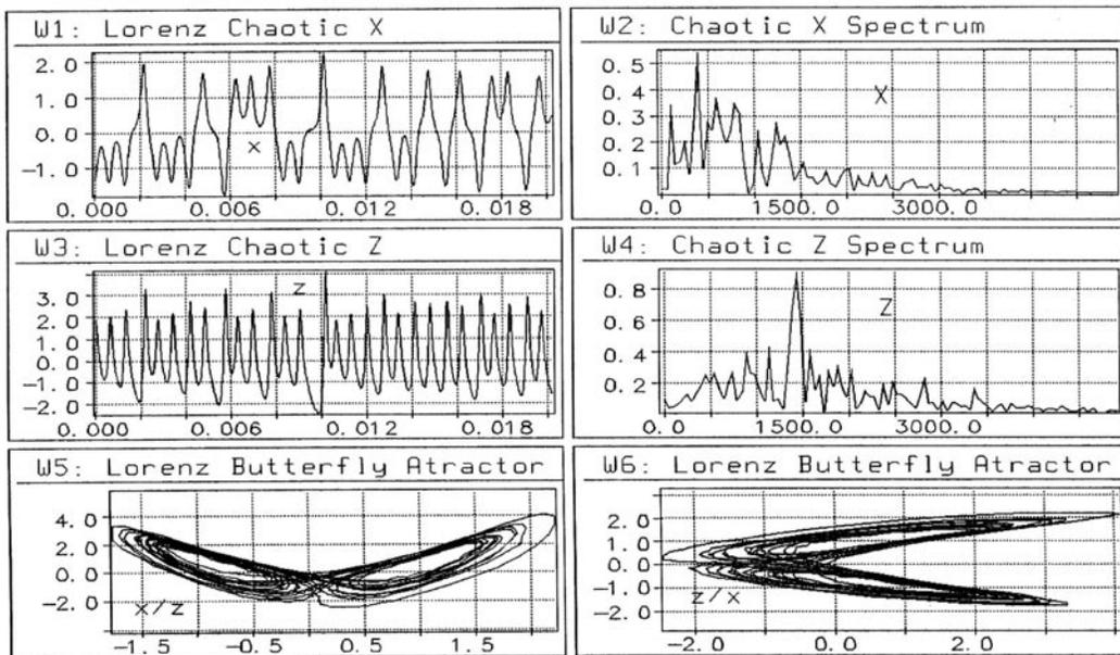
Figure 4. Waveforms, spectra and phase-plans of X and Z; Lorenz Butterfly attractor.
