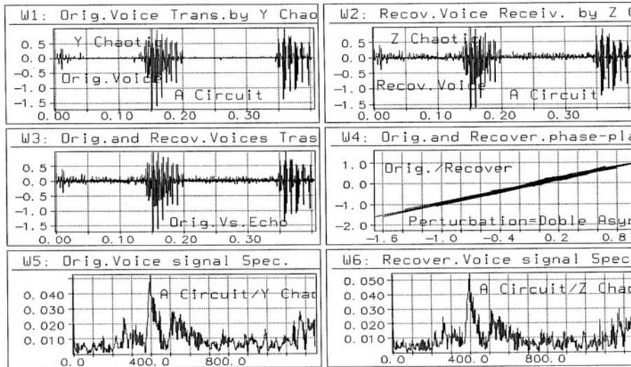
Figure 16. Autotesting the SCBCHI using voice echo signals.
