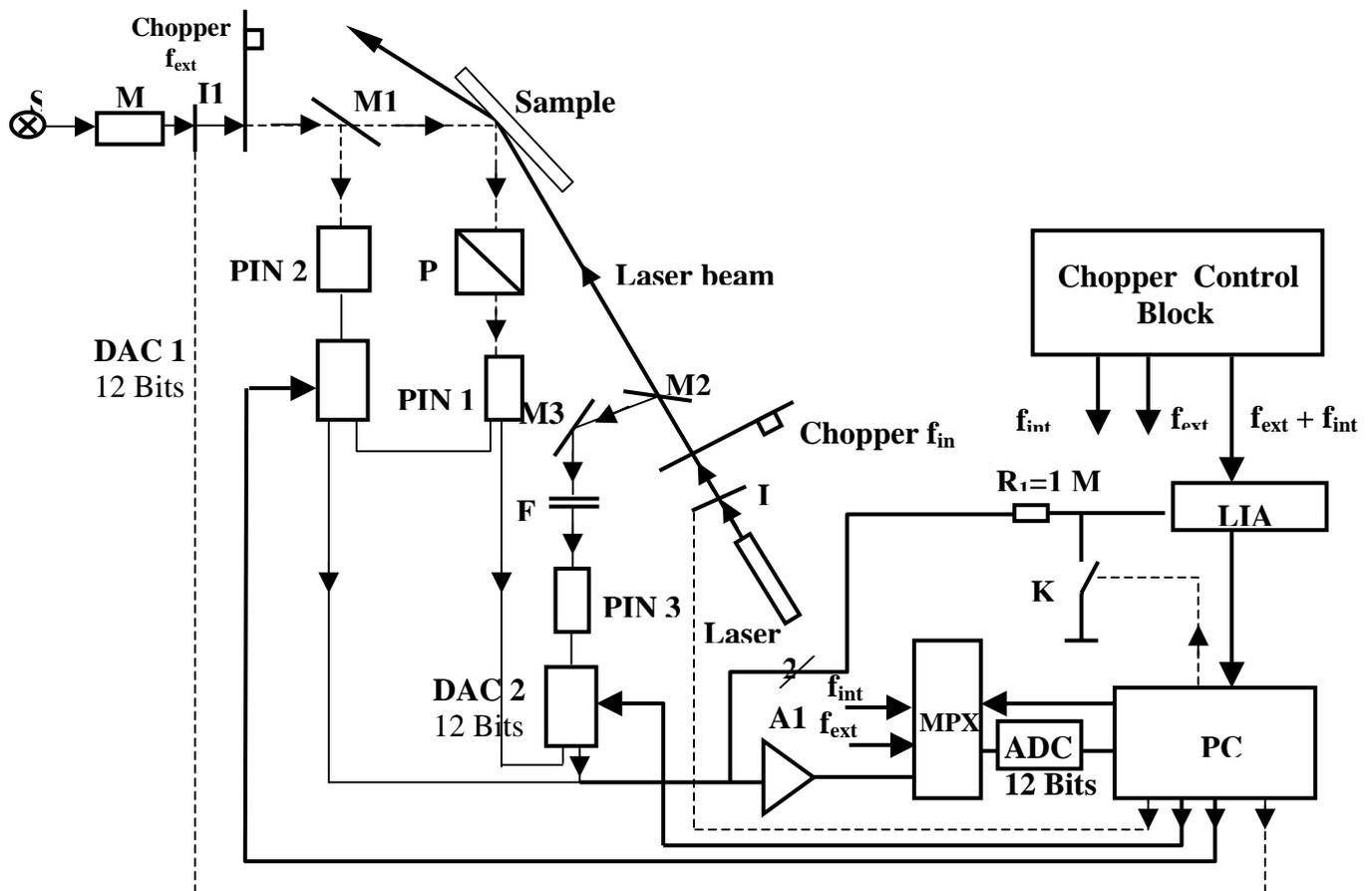
Figure 1. Block diagram of the proposed method
