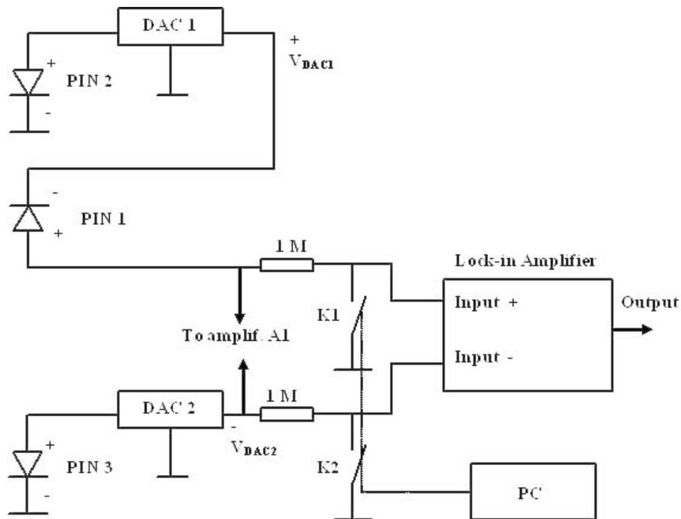
Figure 2. The connection between PIN1, DAC1 and DAC2
