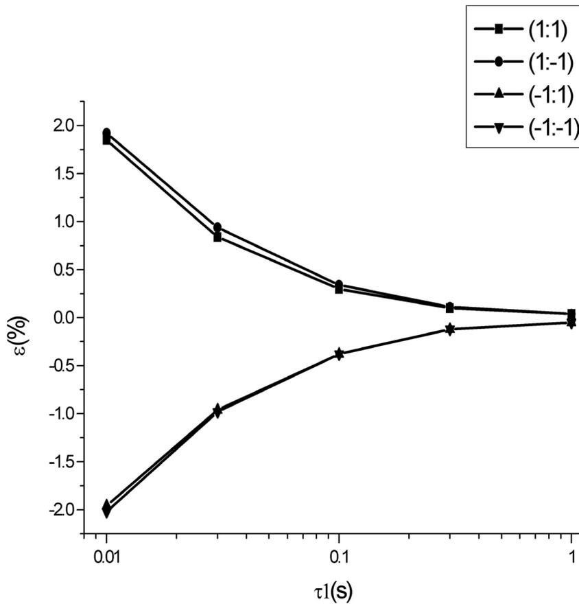
Figure 5. Relative error dependence on the time constant  $\tau_1$  of the lock-in first low-pass filter. The numbers Between the parentheses indicate (monochromator scattered light compensation error; Laser scattered Light compensation error) in LSB
