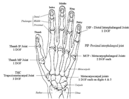
Figure 1. The human hand, the bones that compose it and the DOF belonging to each one of the joints
