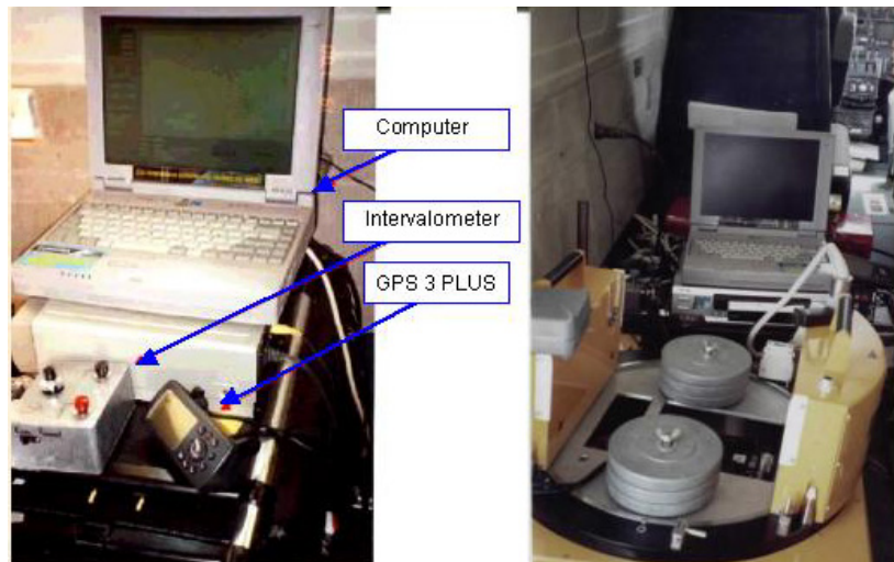
Figure 22. Imaging system with the cameras mounted in the stabilized platform of a Zeiss RMK top aerial camera in a Cessna 441 aircraft.
