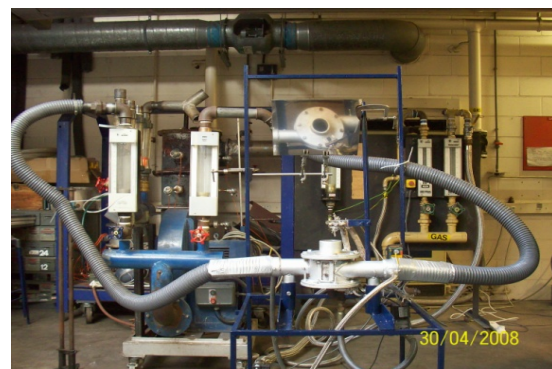
Figure 2. Burner mounted on a rig with a mirror to view the tangential radial plane.
