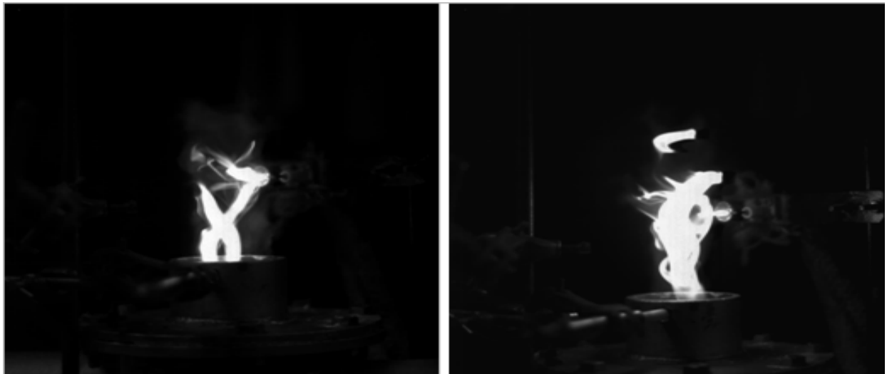
Figure 6. Double PVCs. Pair of strong vortices ( S=2.02 , Re \sim 11,000 , \phi=0.39 ) and main structure surrounded by a bifurcating vortex ( S=1.06 , Re \sim 11,000 , \phi=0.39 ), respectively.
