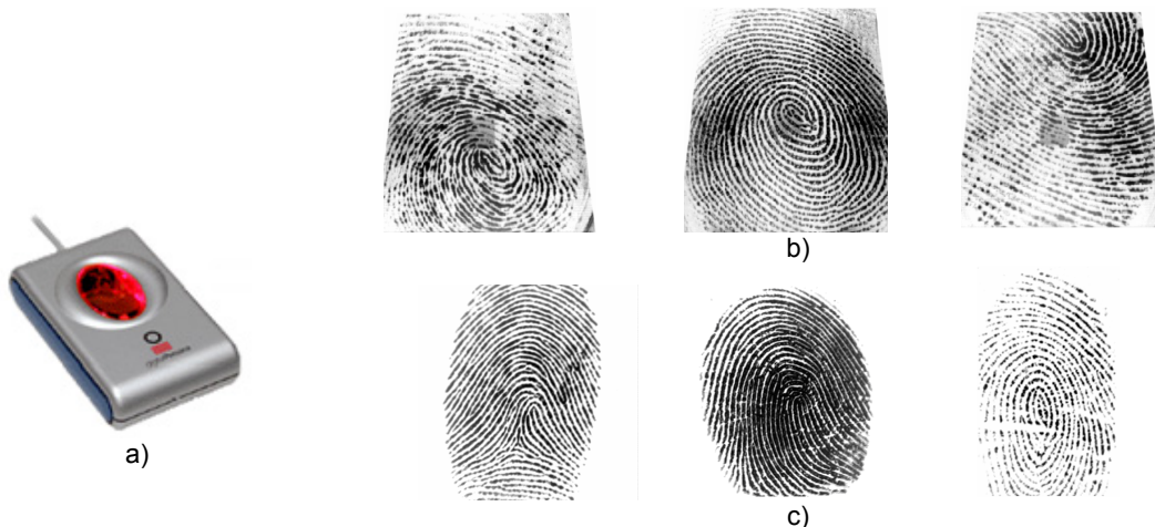
Figure 1. a) Optical reader used. b) Some fingerprint images obtained with the UareU 4000 scanner. c) Fingerprint images obtained from the FVC2002 database
