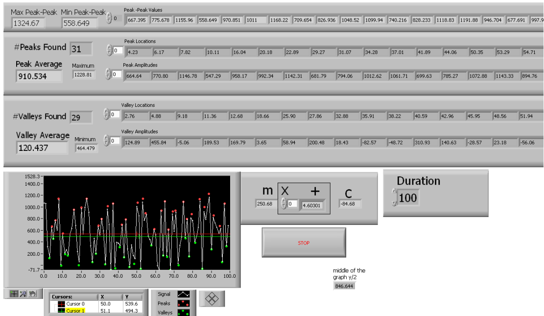
Figure 9. Peak and Valley Detection of ECG wave with its Max. & Min Values.
