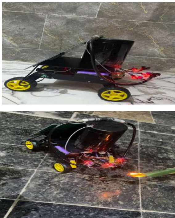
Figure 24. Firefighting robot implementation.
