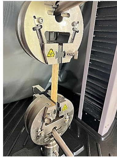
Figure 6. Tensile testing of biocomposites.
