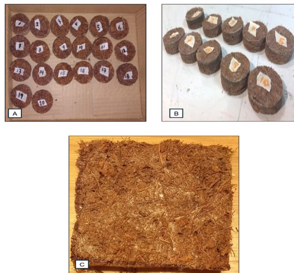
Figure 2. Samples for the acoustic study (coconut fiber-cassava starch-binder): (A) with a high concentration, and (B) with a low concentration. (C) Panel sample for thermal study.
