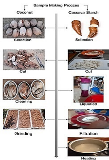
Figure 1. Manufacturing processes to obtain coconut fibers and cassava starch.
