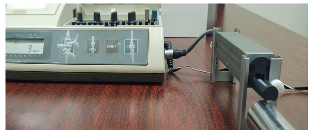
Figure 3. Set up of the roughness tester.
