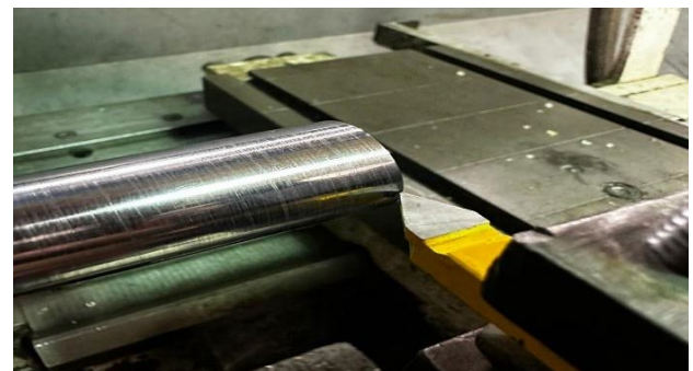
Figure 2. Set up cutting tool on 1018 steel specimen.
