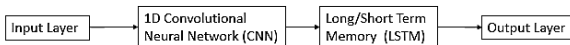
Figure 6. Hybrid method using a combination of 1D-CNN and LSTM architectures for estimating the SoC of Li-ion battery blocks.
