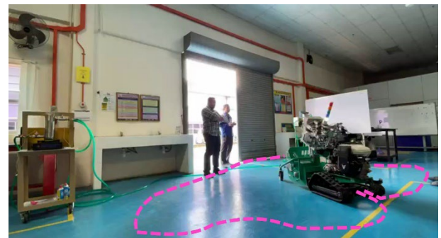
Figure 11. In-lab testing with remote control for path maneuvering and system control testing.
