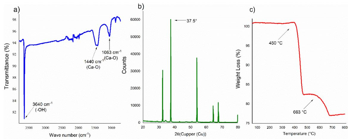
Figure 3. FTIR spectra (a), XRD diffractogram (b), and thermogram TGA (c) for calcined eggshell powder.
