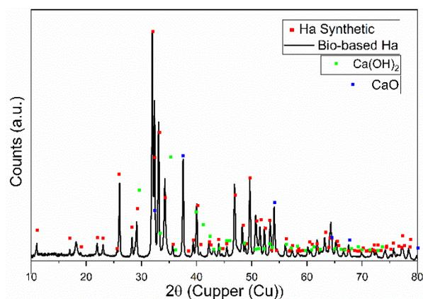
Figure 5. XRD diffractogram of bio-based and synthetic Ha.
