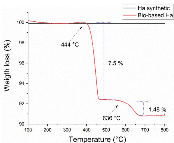
Figure 6. Thermogram of bio-based and synthetic Ha.
