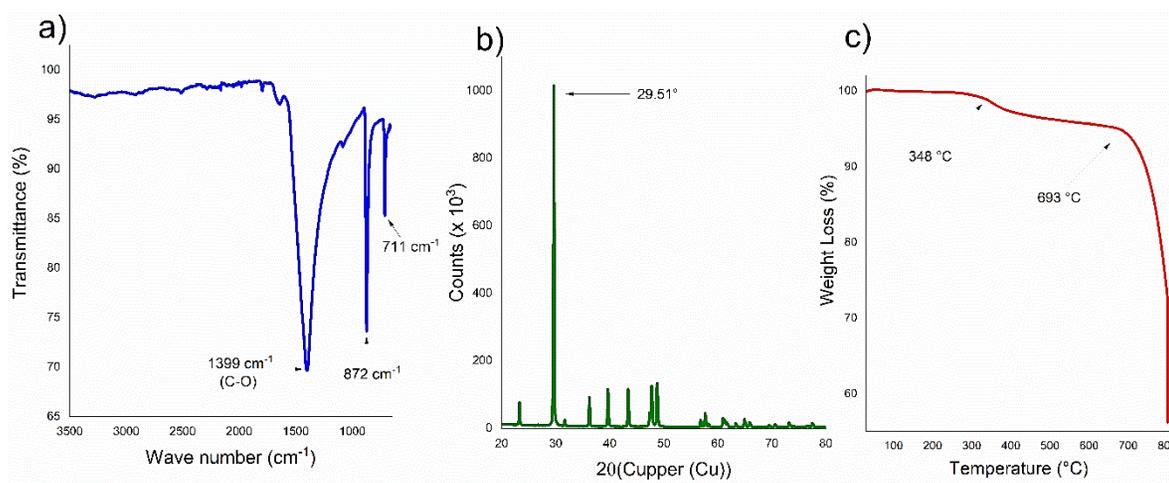
Figure 2. FTIR spectra (a), XRD diffractogram (b), and thermogram TGA (c) for eggshell powder.
