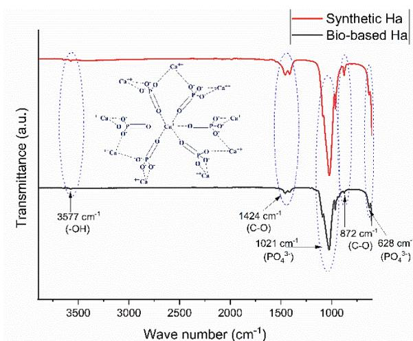
Figure 4. FTIR-(ATR) spectra of bio-based and synthetic Ha.
