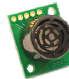
Figure 4. SRF02 ultrasonic sensor model
