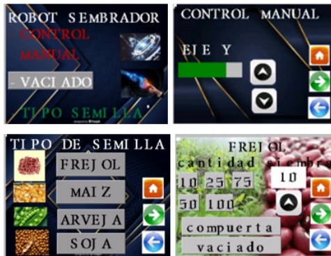
Figure 3. Screens that make up the HMI interface are implemented on the Nextion touchscreen.
