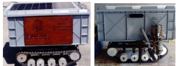
Figure 2. Final exterior view of the mobile crawler robot for seed sowing.
