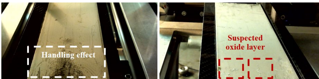
Figure 3. Visual of fuel surface by a dedicated real-time camera.
