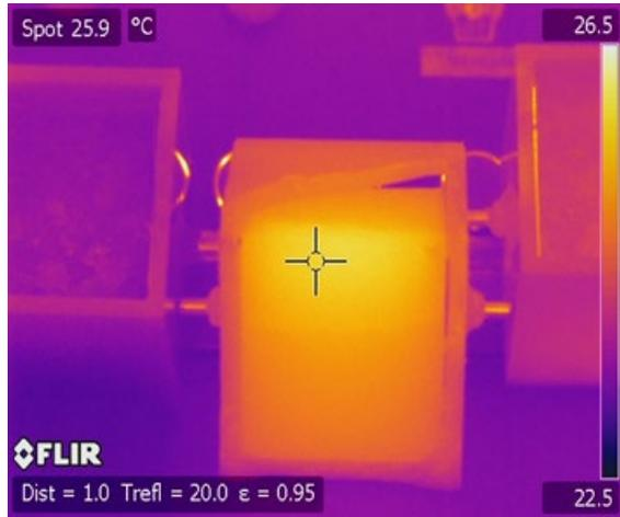
Figure 7. Thermal image of MQ305 sample after lightning impulse current test; it is note that the sample exploded during the last impulse test.
