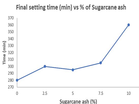
Figure 5. Final setting time versus % of sugarcane ash replacement.
