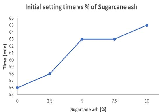
Figure 4. Initial setting time versus % of sugarcane ash replacement.
