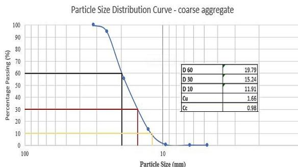
Figure 3. Particle distribution of coarse aggregates.
