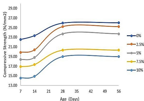
Figure 6. Compressive strength values versus Age of curing.
