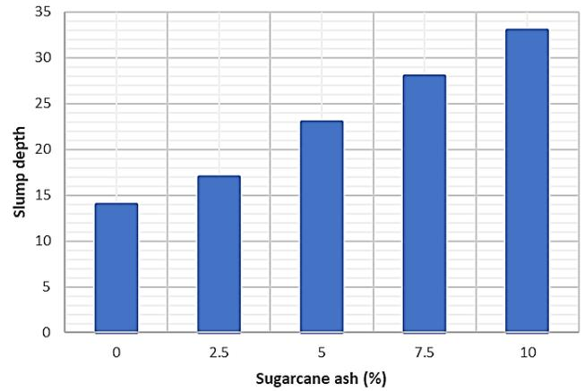
Figure 1. Slump depth versus sugarcane bagasse ash (SCBA).
