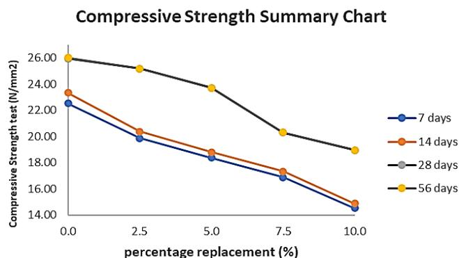
Figure 7. Compressive strength values versus % of SCBA replacement.
