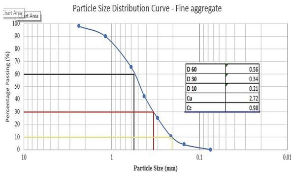
Figure 2. Particle distribution of fine aggregate.
