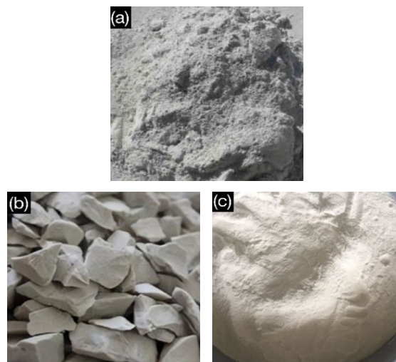
Figure 1. A photograph of fly ash (a), ceramic debris (b), and ceramic waste powder (c).
