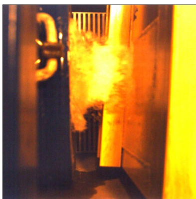
Figure 7. Intense interaction of indenter and ice, ejection of broken ice (t = 0.024 c).
