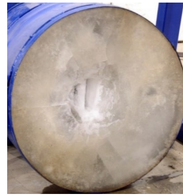
Figure 8. Destruction of ice because of its impact interaction with the indenter.
