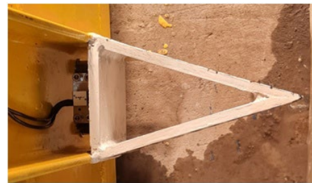
Figure 3. Wedge-shaped indenter with an acceleration sensor.
