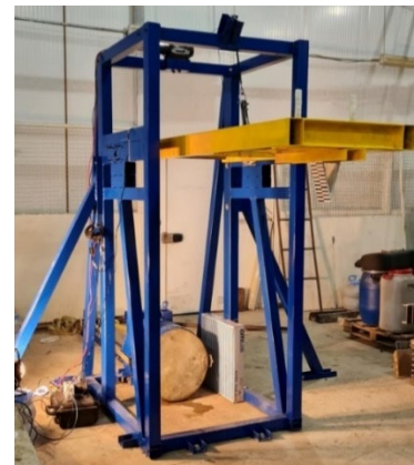
Figure 4. Pendulum impact tester for impact ice breaking.
