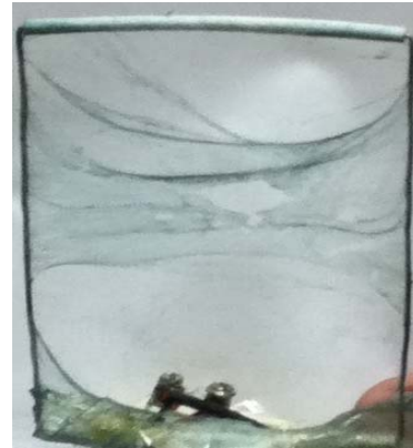
Figure 1. Polyaniline fibers obtained by electrospinning.
