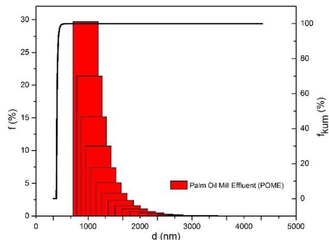
Figure 2. Particle size distribution of nanocarbon from palm oil mill effluent.
