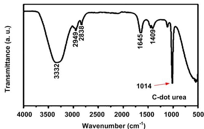
Figure 3. FTIR spectrum of nanocarbon from palm oil mill effluent.
