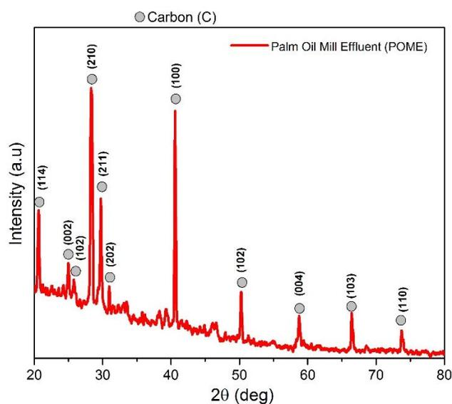
Figure 1. XRD pattern of nanocarbon from palm oil mill effluent.
