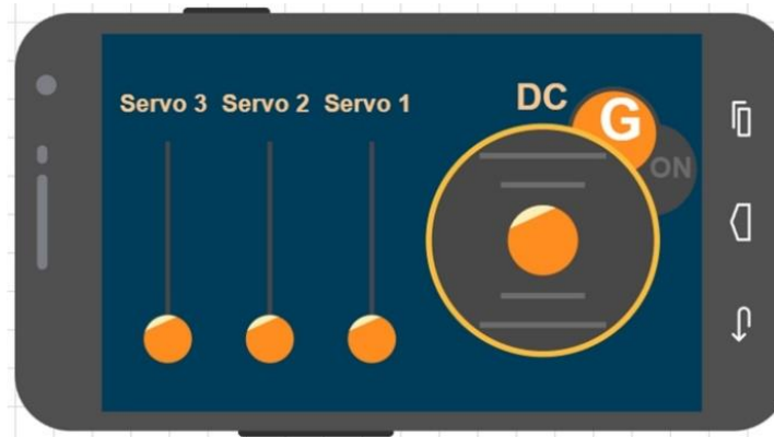
Figure 4. Mobile GUI to control the mobile robot arm.
