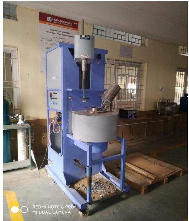
Figure 3. Experimental setup of stir casting process.
