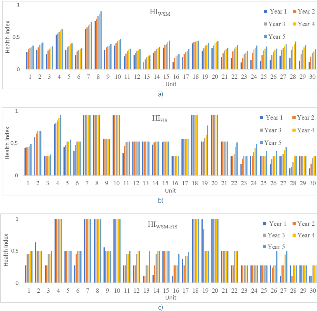
Figure 9 a) to c). Individual comparison for the three methods for the five-year period. a) Health index based on a weighted sum model. b) Health index based on fuzzy inference system. c) Health index based on hybrid WSM-FIS.
