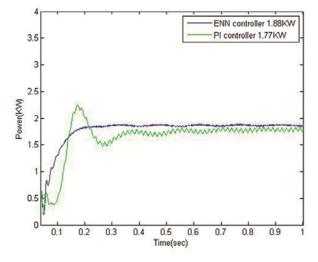
Figure 8. Maximum power tracking response of the WECS.
