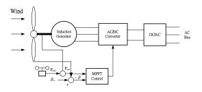
Figure 6. Configuration of the wind-generation system.
