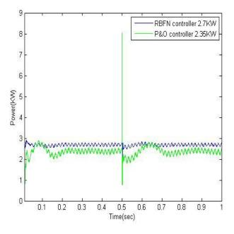
Figure 11. PV power generation in load varied condition.
