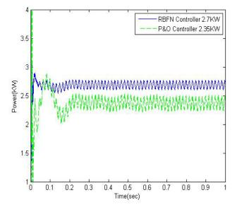
Figure 9. Power response of the PV system.
