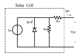
Figure 2. Equivalent circuit of a PV cell.
