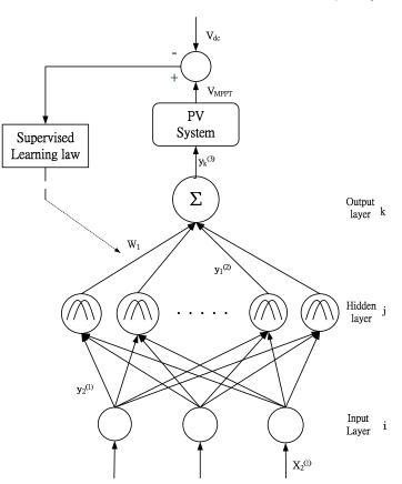
Figure 5. Structure of the three-layer RBFN.
