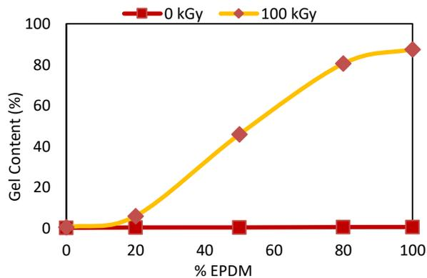
Figure 2. Gel content of PP/EPDM binary blends.
