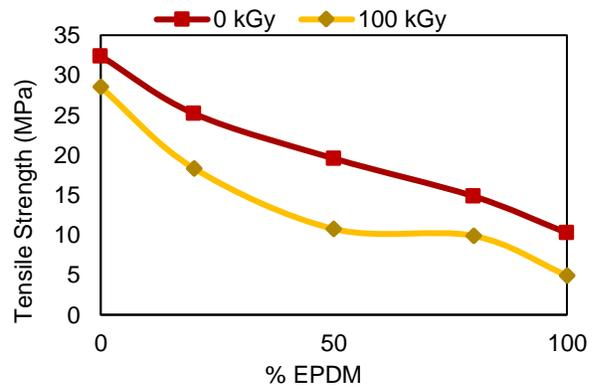
Figure 4. Tensile strength of PP/EPDM binary blends.
