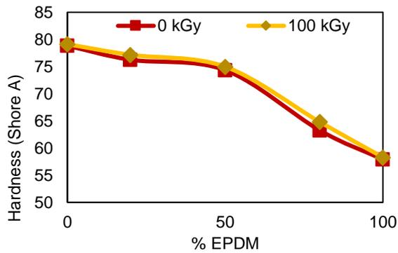
Figure 8. Hardness of PP/EPDM blends.
