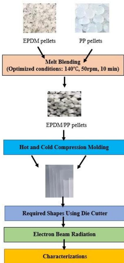
Figure 1. Preparation of PP/EPDM binary blends.
