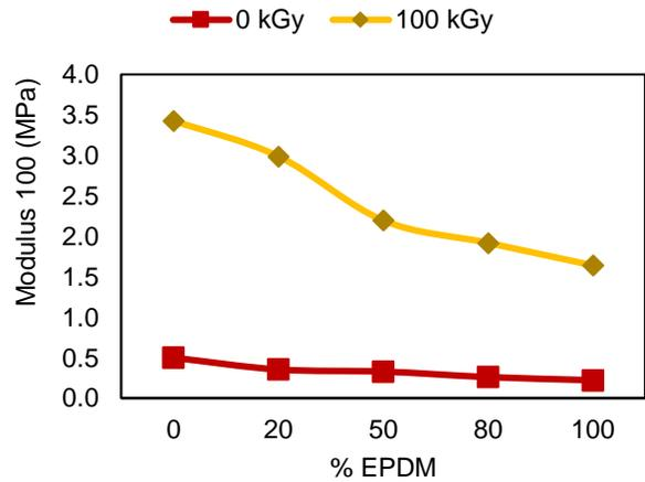
Figure 6. Modulus 100 of PP/EPDM binary blends.
