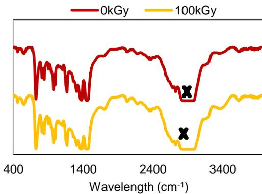
Figure 3. FTIR of PP/EPDM binary blends.
