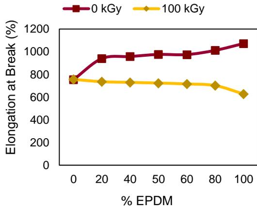
Figure 5. Elongation at break of PP/EPDM binary blends.
