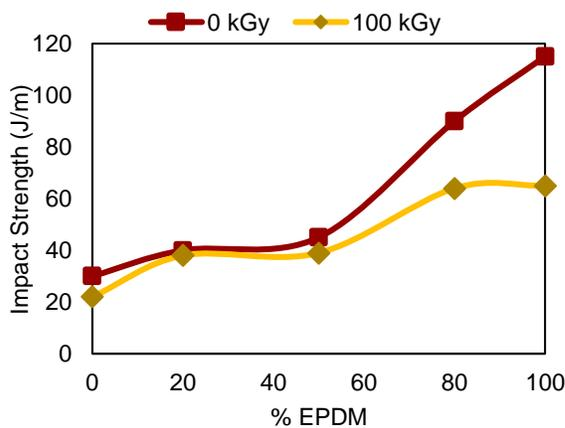
Figure 9. Impact strength of PP/EPDM binary blends.
