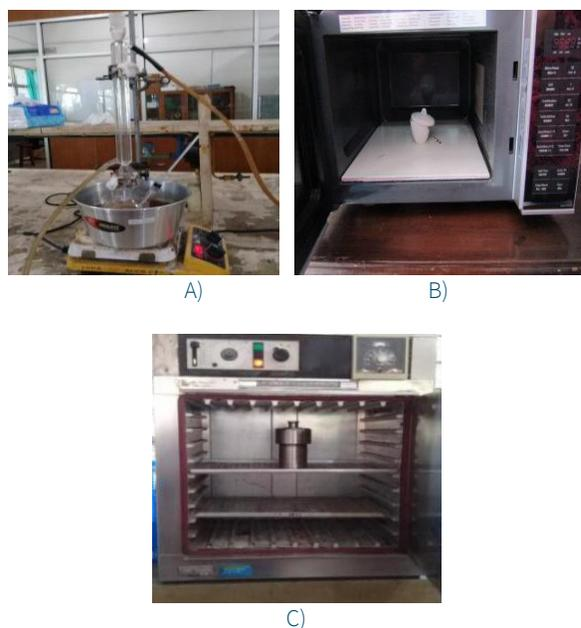
Figure 1. Tools for pyrolysis: A) Reflux, B) Microwave with porcelain crucible, C) Oven with autoclave.
