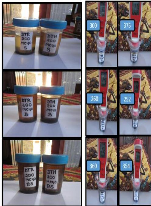
Figure 14. The CNS colloids prepared using the reflux-microwave (DTR200-MC40) and the hydrothermal - microwave (DTH200-MC40) and TDS measurements using mini TDS meter.
