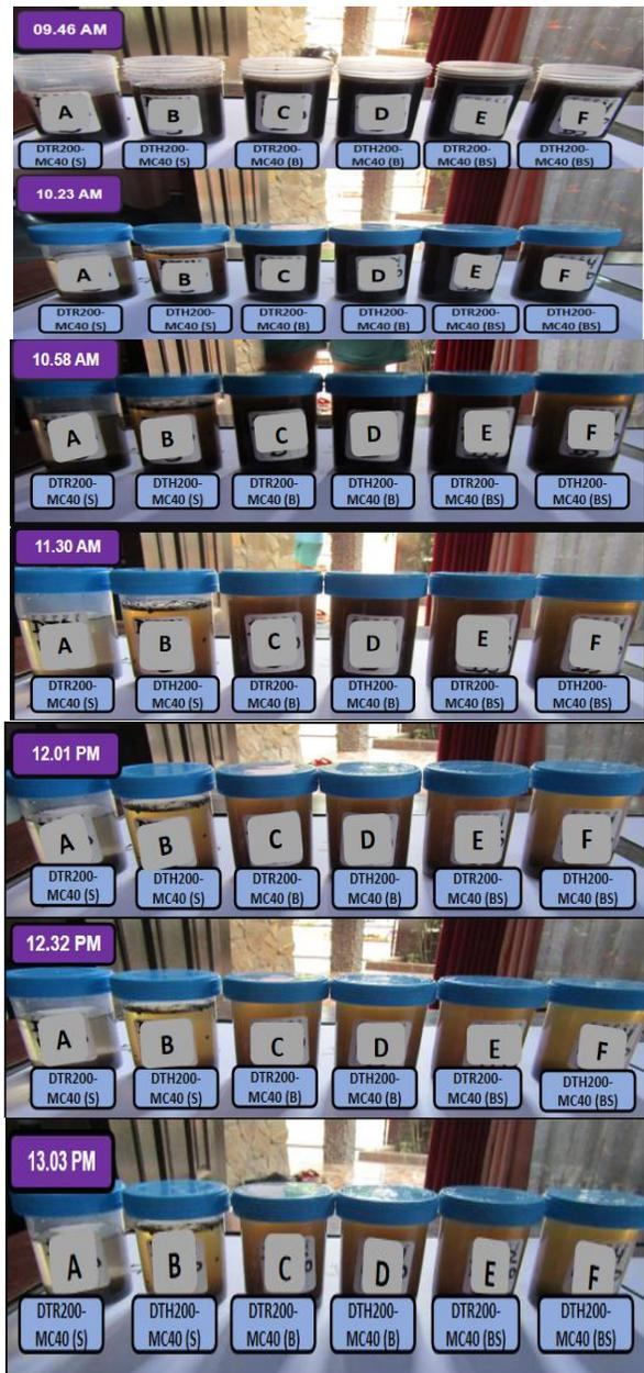
Figure 12. Test of nanocarbons dispersion stability by techniques of sonication (S), blending (B), and blending - sonication (BS).
