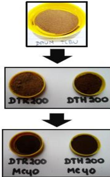
Figure 3. Biomass (DT) and pyrolyzed biomass by reflux (DTR200), hydrothermal (DTH200), reflux - microwave (DTR200-MC40), and hydrothermal - microwave (DTH200-MC40).
