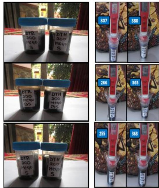
Figure 13. The CNS colloids prepared using the reflux-microwave (DTR200-MC40) and the hydrothermal - microwve (DTH200-MC40) and TDS measurements using mini TDS meter.
