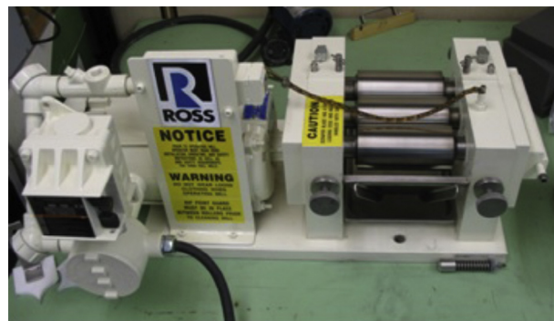
Fig. 1. Ross three-roll-mill used to make CNT-grease.
