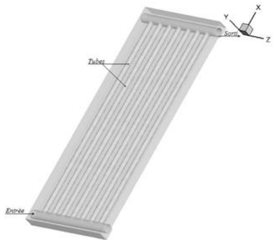
Figure 2. Geometry of a solar collector equipped with seven parallel tubes over an aluminum absorber and a simple white glass cover.
